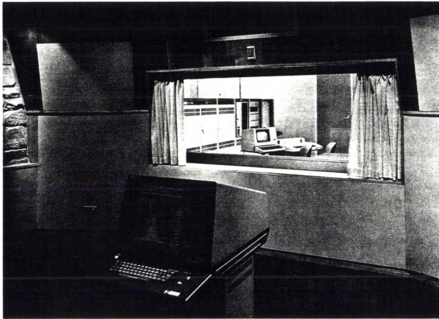
Fig. 38. The computer (visible through the window) can perform various functions in designing digital filters. Besides making all kinds of design calculations and displaying the resultant filter characteristics on a screen (foreground) the computer can immediately simulate the result that a particular filter would give in practice. The foreground in this photograph is a 'listening room', which is almost completely isolated acoustically from the environment. The effects of digital signal processing on audio signals can be assessed in this room by using simulated signals.
