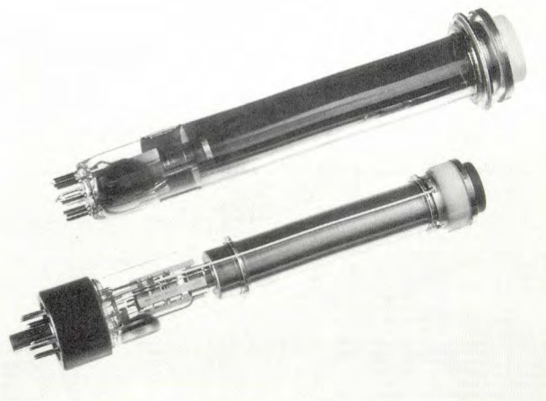
Fig. 11. 1-inch and 2-inch Plumbicon tubes. The Plumbicon tube replaced the vidicon and solved the problem of excessive inertia. Enlargement of the photosensitive area enabled the number of lines in the frame to be doubled, thus greatly increasing the picture definition. This was turned to great advantage in digital imaging techniques.
