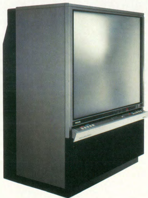
Fig. 16. Modern projection-television set. It contains three separate 7-inch high-resolution cathode-ray tubes, which each reproduce a sub-picture in one of the basic colours red, green and blue. The three sub-pictures are projected on the screen under electronic control to give exact registration. The actual screen is rectangular and flat with a diagonal of 37 inches (about 94 cm). Below the screen there is a drawer (shown open) containing various controls for vision and sound. The set can also be operated with remote control.
