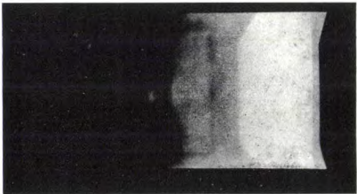
Fig. 4. Photograph of the opal glass in the model of the old hall (fig. 1a). The stage is on the right-hand side. The rapid diminution in illumination intensity towards the left may be noted: at the rear of the hall the useful sound intensity was far too small. The bright trapezoidal spot near the stage is due to reflection at the forefront of the ceiling which was not screened by the transverse roof trusses.
