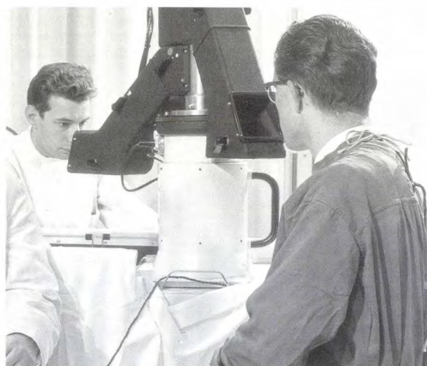
Fig. 6. The Alfalix, an X-ray image intensifier with a diameter of 9 inches, equipped with double mirror optics and a cine camera. During fluoroscopy two observers (e.g. radiologist and surgeon) could examine the image at the same time and film it when required.
