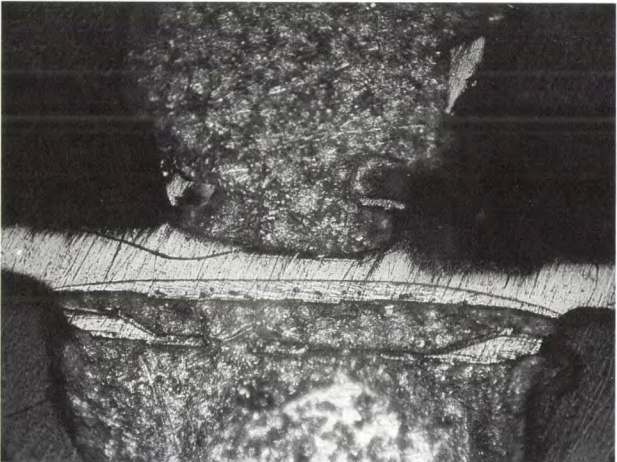
Fig. 3. Germanium junction transistor made by the alloy method. In applying each of the p-n junctions an indium bead or pellet was melted with the germanium, resulting in a recrystallized p-type region after cooling. The problem with this pnp alloy transistor was accurate control of the distance between the two p-type regions (the base width).
