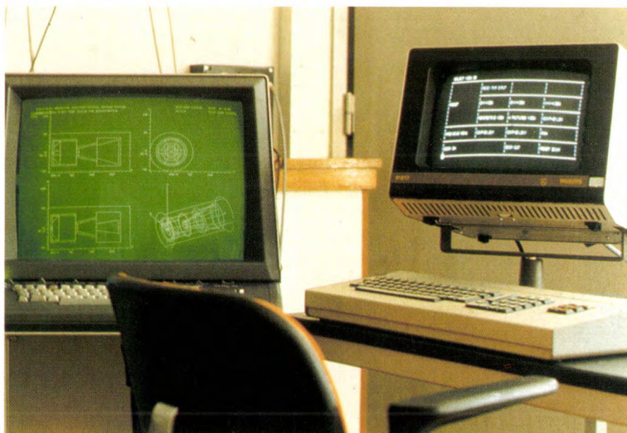
Fig. 2. The GELOP terminal. Left, the graphic display, right, the alphanumeric screen. 'Menus' displayed on the alphanumeric screen enable the user to make his wishes known to the computer system. The results of the calculations are displayed on the graphic display.
